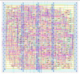
Fig. 5. The physical design of the final IC
