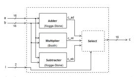
**Fig. 3.** Block diagram of the proposed design of the Fixed Point Arithmetic Unit.
