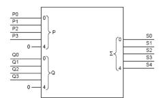
**Fig. 1.** Example of an N+1 bit adder to perform N bit unsigned addition for N=4.
