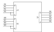
**Fig. 2.** Example of an N+1 bit adder to perform N bit signed addition for N=4.
